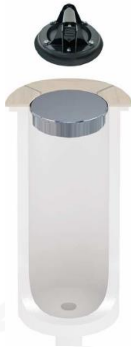
Fig. 1 REMOVAL OF EMBEDDED COVERPLATE FROM FOUNDATION
