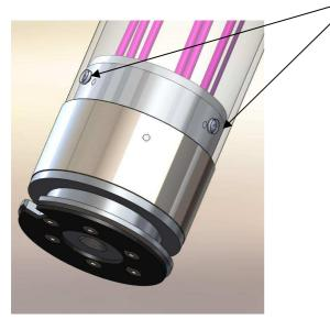
4.) unscrew both screws, remove cover and block from output and unclip spinlock
